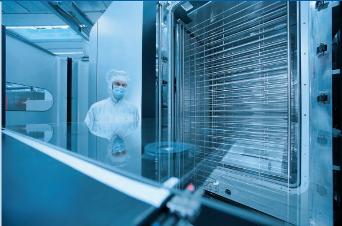
Fig. 4 - Unaxis Solar KAI 1200 mass production system for thin film silicon solar modules (photo Unaxis).
